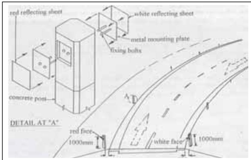
Figure 5: Post delineator and its installation
