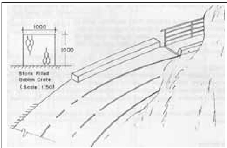
fig. 9: Gabion barrier
