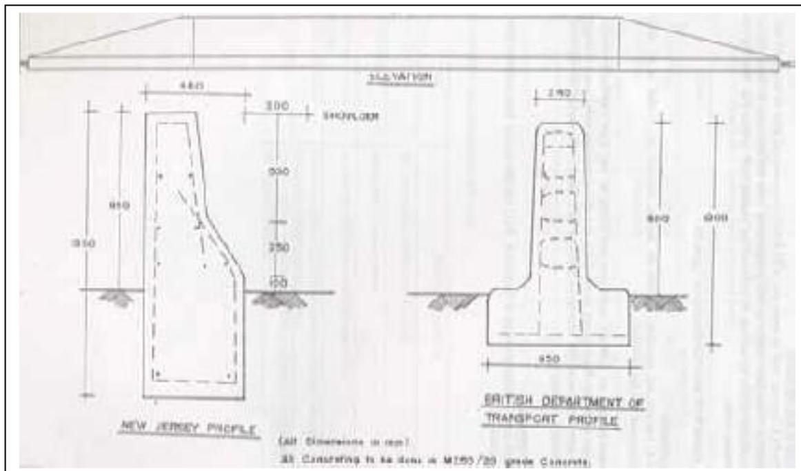
Fig.12: Alternate types of RCC barrier
