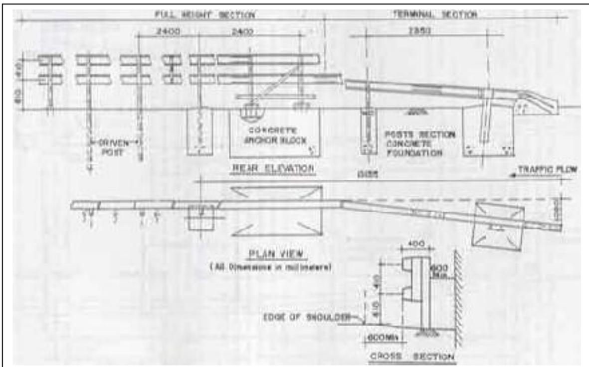
Fig.8: Open box beam barrier – double railed and untensioned (Adapted form UK Highway Construction details, Vol 3, Section 2)
