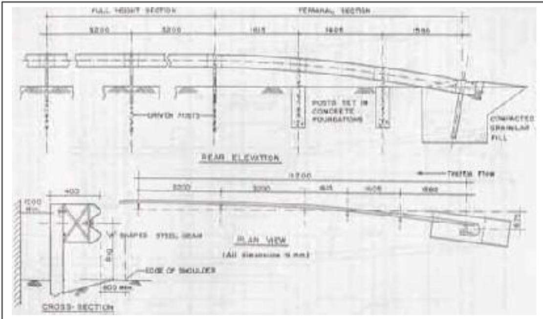
Fig.7: Corrugated steel beam barrier – untensioned (Adapted form UK Highway Construction details, Vol 3, Section 2)
